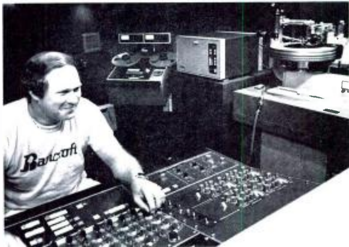
Seated at a Neve disc-mastering console at Filmways/Heider studios, engineer Phil Cross oversees a tape-to-disc mastering session. Between the lathe and an Ampex ATR-100 is the new Ampex ADD-1 digital delay system.
